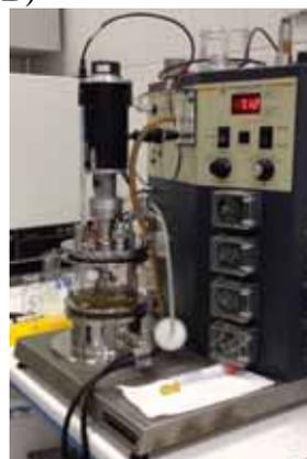
Figure 1. A) Progress curve of cholecalciferol (black line) hydroxylation to calcifediol (blue line), B) pilot semi-technical reactor installation used in the synthesis equipped mechanical mixer, thermostat and pH control.
