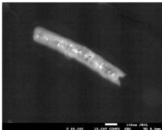
Figure 1. SEM picture of the carbon nanotube filled with \text{Ce}(\text{NO}_3)_3 . Picture was made in the "compo" mode (reflected electrons). In that mode of acquisition the brightness of the pattern is proportional to z^2 , where z is the atomic number of the atoms constituting the sample surface. Because cerium has much higher atomic number than carbon, regions rich in cerium look bright. Presented pictures strongly suggest that cerium was located inside the carbon nanotubes
