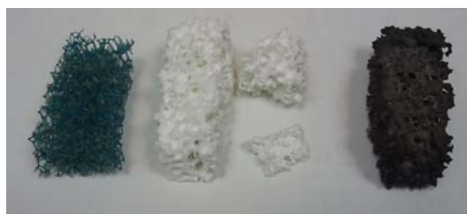
Figure 1. Polyurethane foam, sintered ceramic foam and ceramic foam catalyst (from left to right)
