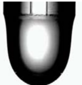
Profile of the pendant drop for surface tension measurements by drop shape analysis
