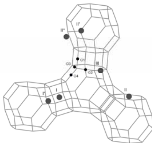
Possible cation positions (grey balls) and different O crystallographic positions (black balls) in FAU.
