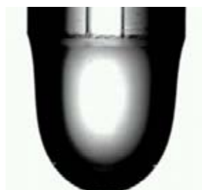
Profile of the pendant drop for surface tension measurements by drop shape analysis
