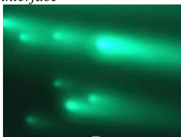
Release of fluorescent dye from microcapsules attached to a surface
