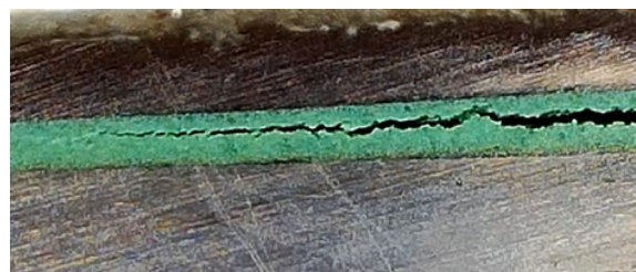
Fig. 2 Microscopic image of a 290 μm thick malachite paint film during the test. Thin dark areas of adhesive penetration are visible at both film surfaces. The crack grew in the paint material not penetrated by the adhesive
