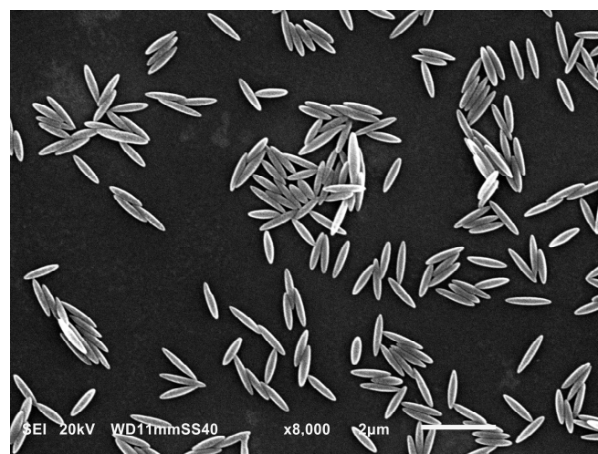
Figure 2. The SEM micrograph of the P(S/PGL) particle layer.
