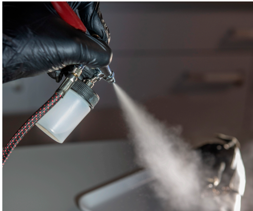
Figure 2. Application of ethanol mist with antibiotics using an airbrush.
