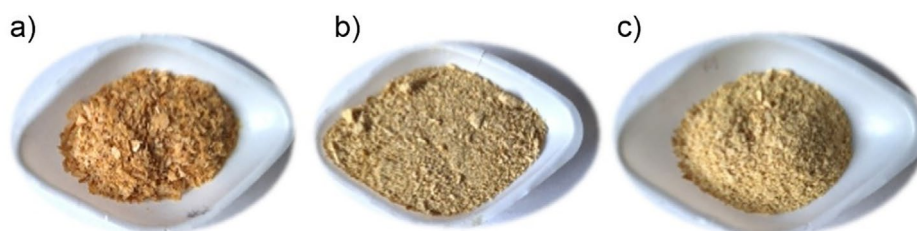
FIGURE 1 | Dried bacterial biomass samples used in this study for the extraction of PHAs. (a) Z. denitrificans MW1, (b) MMC and (c) P. putida CA3.
